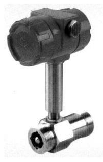
LWGB type turbine flow sensor is on the basis of LWGY prototype turbine flow sensor increased the 24 VDC power supply, two wire system 4-20 ma current transmitting function, especially suitable for computer, such as display, industrial control, DCS control system.
