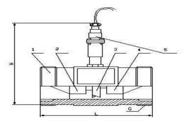
1. Shell 2. Front guide piece 3. Impeller 4. Behind guide piece 5. Pre-amplifier
