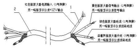
Figure 4 sensors and display instrument wiring schematic diagram
